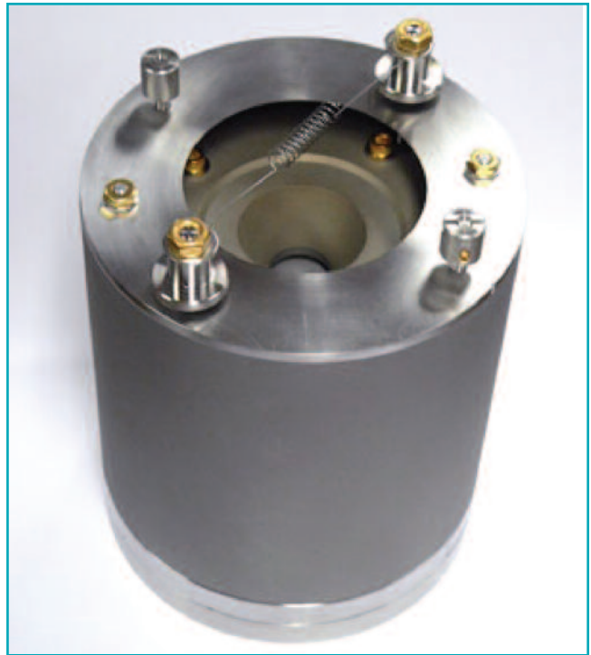
Figure 4a. Mark-2 end-Hall ion source with a Tungsten HF (in a form of spiral) electron source produced by Veeco Instruments.
